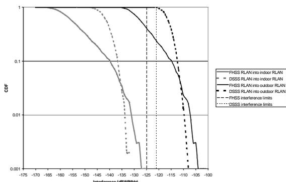
**Figure 3. Interference CDF plots when the interference is caused by indoor RLANs**
