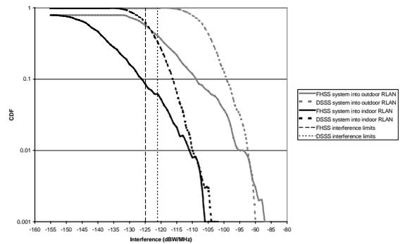
**Figure 2. Interference CDF plots when the interference is caused by outdoor RLANs**
