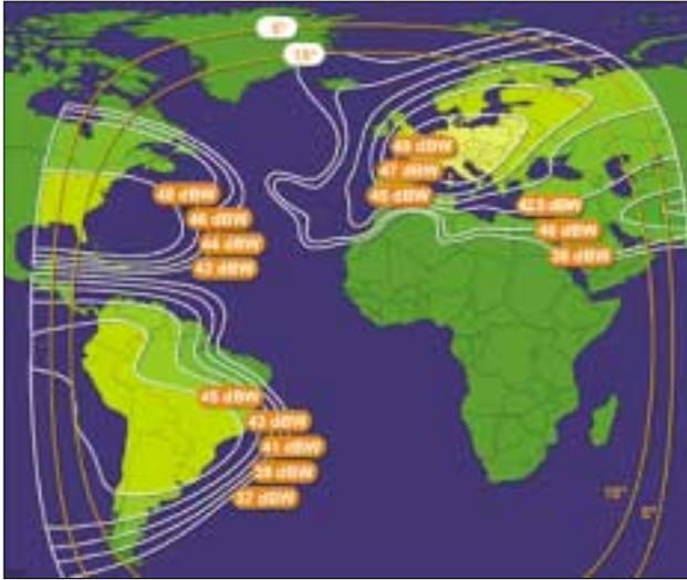
Fig. 1 Multibeam satellite downlink coverage
