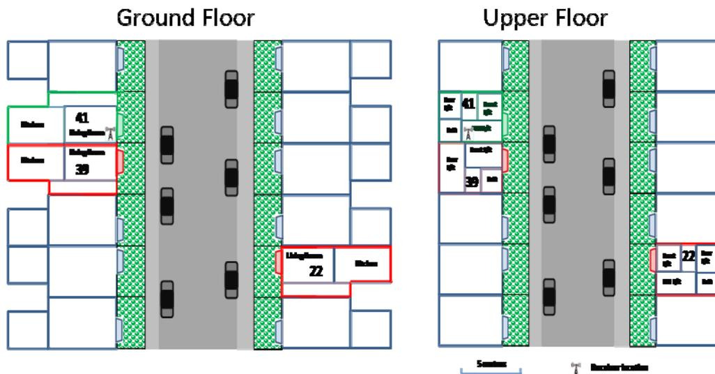
Two series of measurements were taken, one with the spectrum analyser located by the front window of no.41 and the other taken with the analyser located in the attic room of number 41. Measurements were undertaken at two frequencies, namely 2400 MHz and 498 MHz, operating under a non-operational licence issued by Ofcom.
