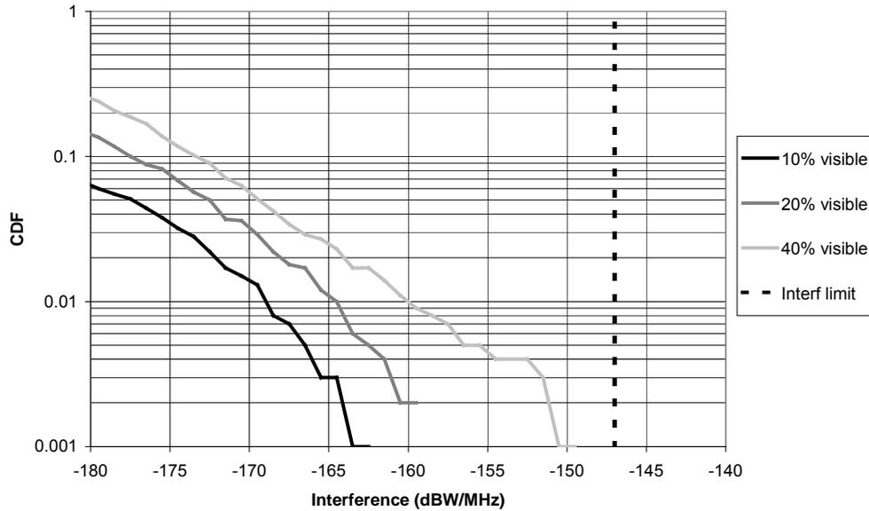
**Figure 3.16: CDFs for subscriber station to base station interference (geographically adjacent PMP networks)**
