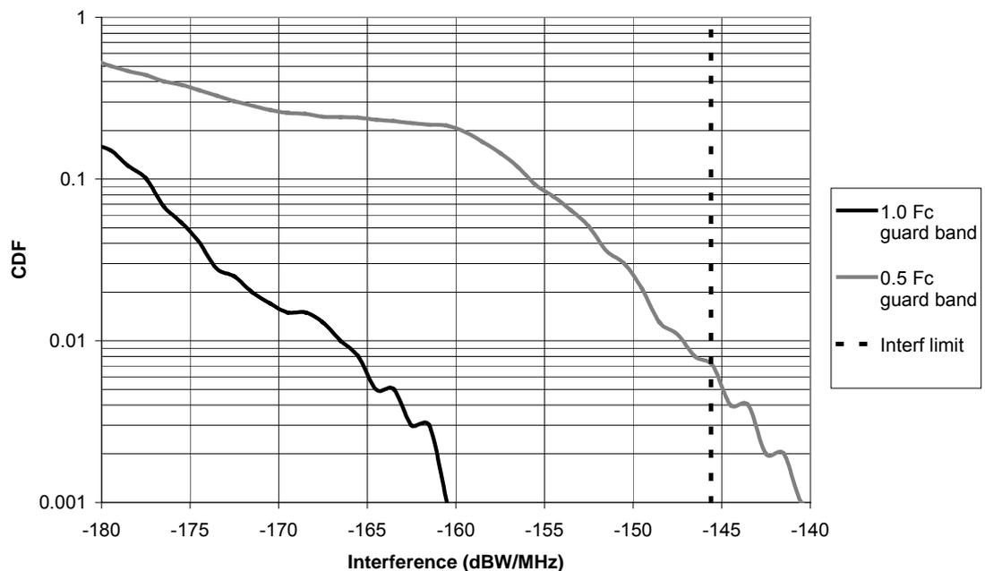
**Figure 4.8: Interference between PMP base stations (interferer density 0.009 per km<sup>2</sup>)**
