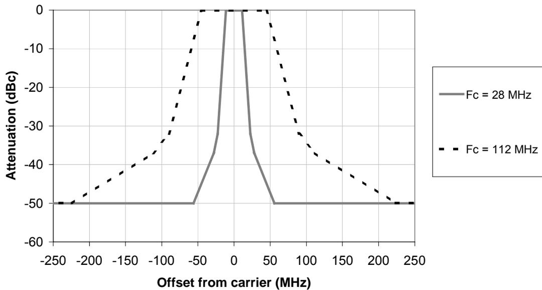
**Figure 2.4: Comparison of transmission mask roll off for 28 MHz and 112 MHz systems (based on EN 301-213, TDMA type B)**
