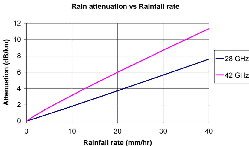
**Figure 2.7 Comparison of rain attenuation at 28 GHz and 42 GHz**
