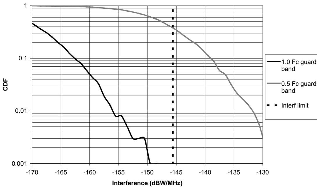
**Figure 4.10: Interference between high density mesh network and PMP base station (interferer density 0.45 per km<sup>2</sup>)**
