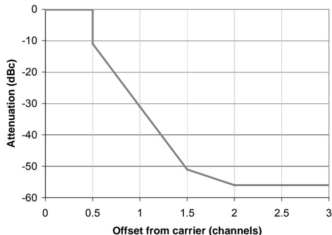
Figure 2.5: FCC spectrum mask
