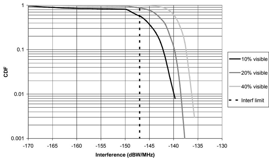
**Figure 3.11: Interference CDF for base station to base station scenario (no base station antenna down tilt)**
