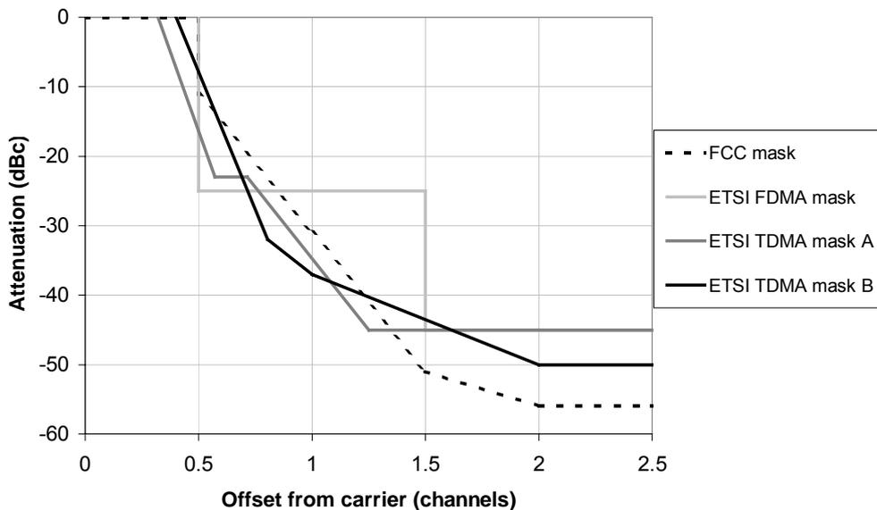
**Figure 4.2: Transmitter spectrum masks defined in EN 301 213**
