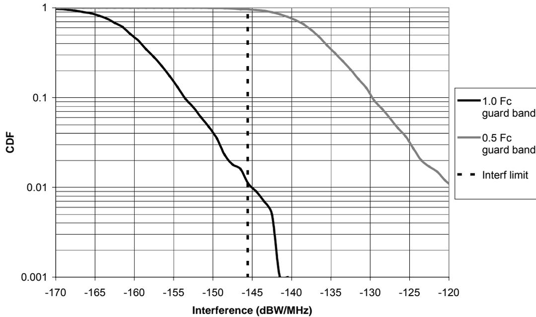
**Figure 4.11: Interference between high density mesh networks (interferer density 0.45 per km<sup>2</sup>)**
