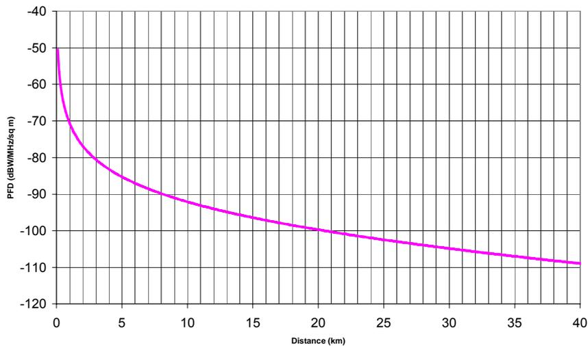
**Figure 3.3: PFD vs. distance from interfering transmitter (0.5 dBW/MHz interferer EIRP)**
