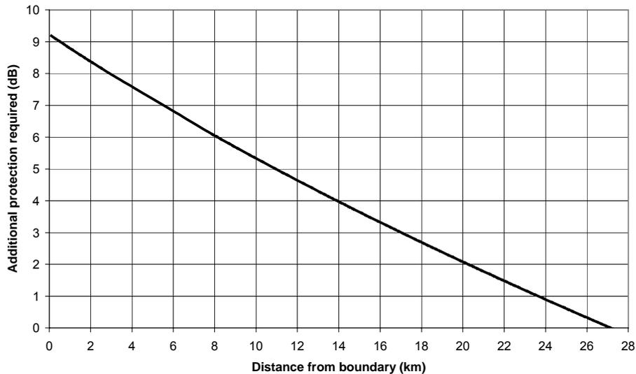
**Figure 3.9: Additional shielding or off-axis discrimination required for base station as a function of distance from service area boundary (28 GHz band)**
