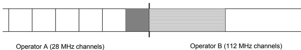
**Figure 4.7: Use of different channel spacings in adjacent bands**
