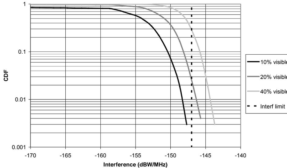
**Figure 3.12: Interference CDF for base station to base station scenario (9° base station antenna down tilt)**
