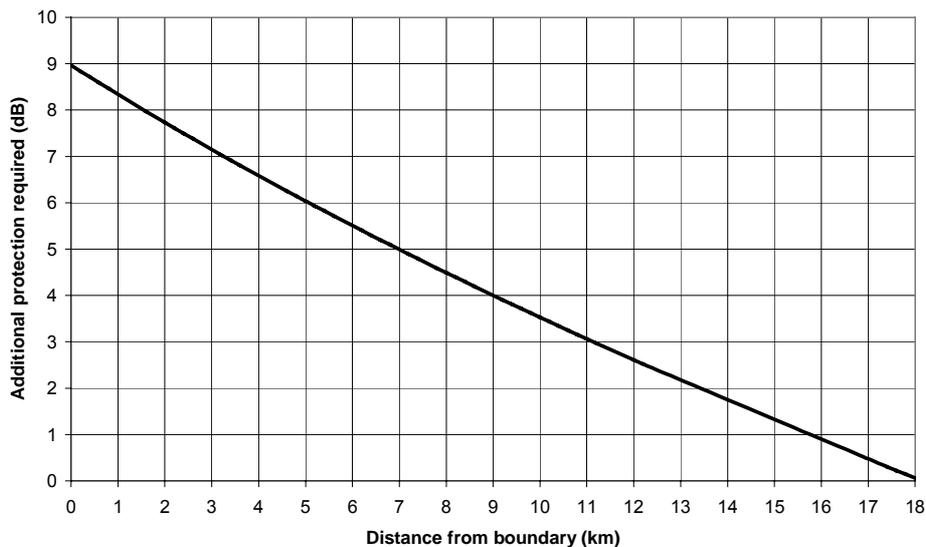
**Figure 3.4: Additional shielding or off-axis discrimination required for base station as a function of distance from service area boundary (42 GHz band)**
