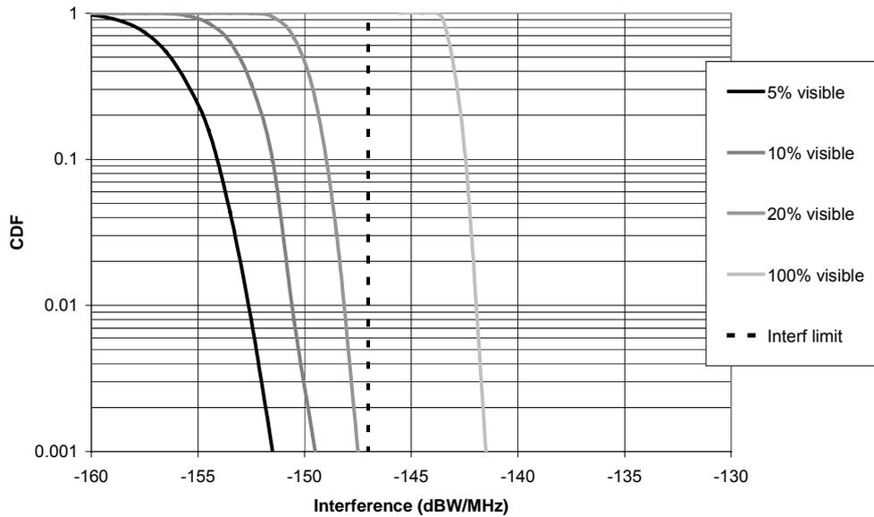
**Figure 3.17: CDF for interference from a high density mesh network into a PMP base station (no co-channel operation within 5 km of service boundary)**
