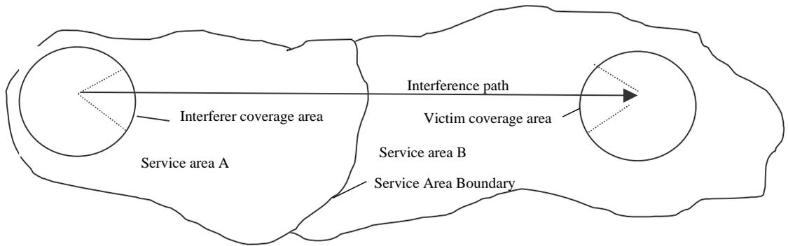
**Figure 3.1 Base station to base station interference scenario**
