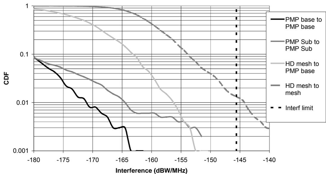
**Figure 4.6: Interference CDFs between networks using identical channel spacings**
