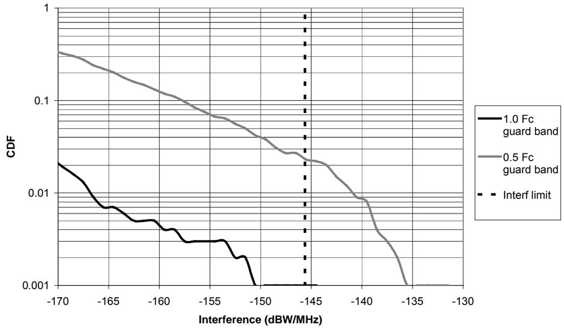
**Figure 4.9: Interference between PMP subscribers (interferer density 0.009 per km<sup>2</sup>)**
