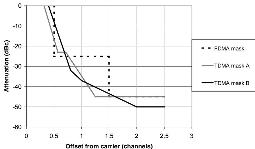
Figure A.1: EN 301 213 transmitter spectrum masks
