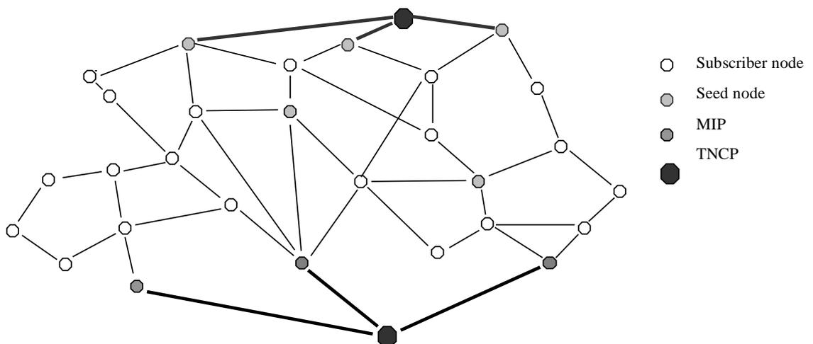
Figure 2.6: Illustration of Radiant Networks mesh architecture
