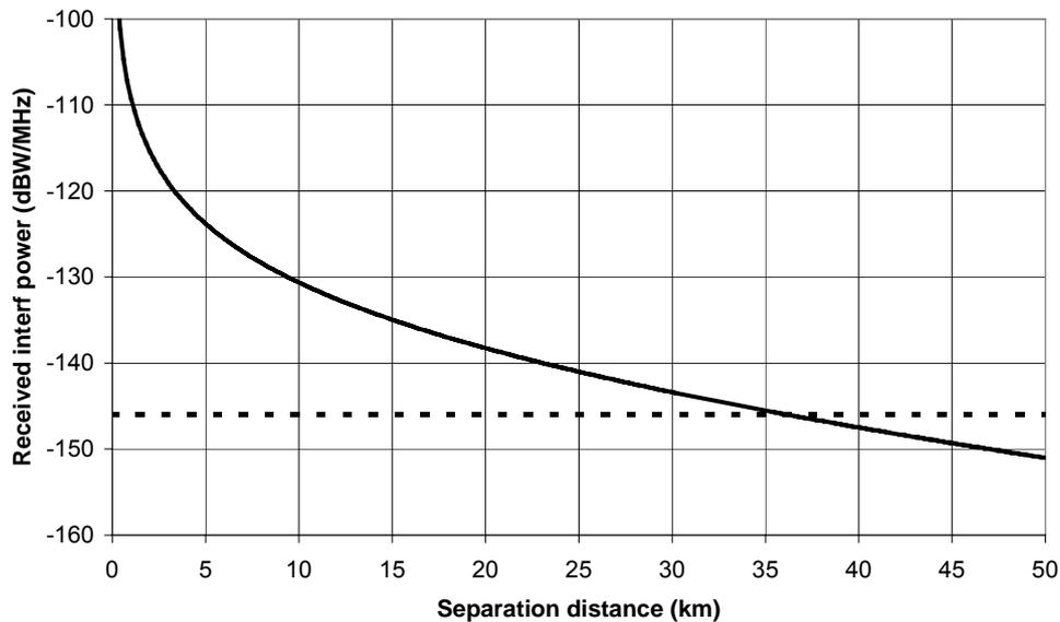
**Figure 3.2: Received interference power vs. separation distance for the base station to base station interference scenario (40.5 GHz, line of sight)**
