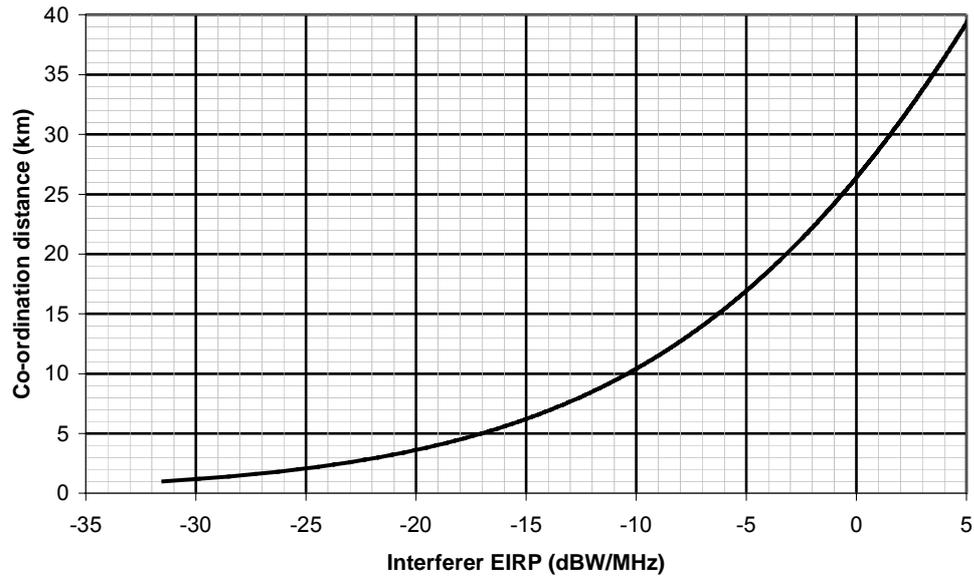
**Figure 3.8: Co-ordination distance from service area boundary as a function of transmitter EIRP) at 27.5 GHz**
